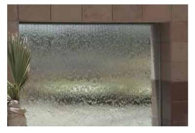
A highly effective nozzle which gives an even distribution of water across walls of any surface leaving a thin film of water to shimmer down the wall. Light these up with LED strip lights for an even more spectacular yet elegant look.
